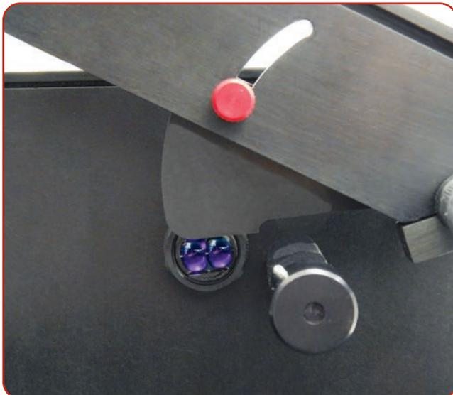
Optical shut-off sensor with adjustable stop
